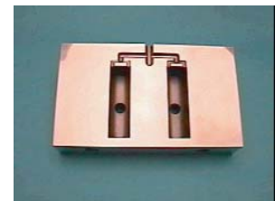
Photograph of a die made with conformal cooling using the LENS process
