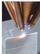
Photograph of LENS process in operation. A laser is used to melt a thin surface layer of material, and powder is injected into the molten pool through four copper nozzles in order to make components in a layer-by-layer fashion.
