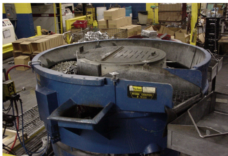
Installed Spiratron “Roto-Finish” Vibratory De-Burring Machine in Vibe Room
