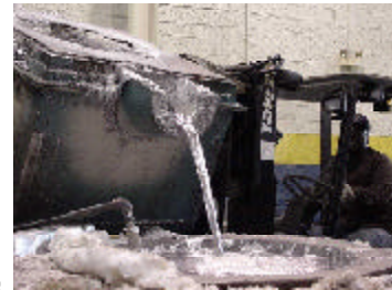
Marcuss Burgess replenishes metal at a die casting machine.
